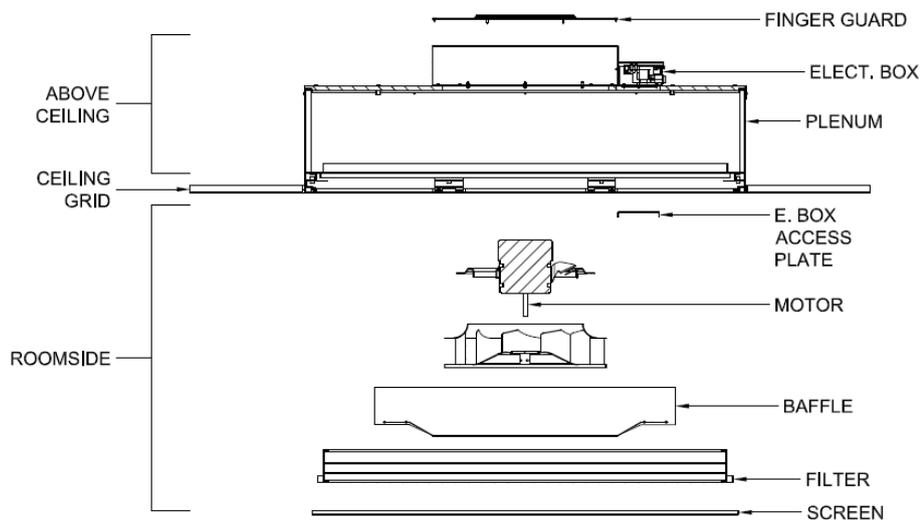
Room-side filter, motor, and electrical components configuration above. The screen, filter, baffle, motor assembly, and electrical components can be removed from the room-side. All other components are only accessible from above the ceiling.
