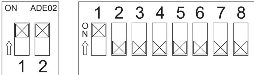
**Note: Network mode can be configured using either DIP switch setting shown above. DIP switch pictorials are for reference and may be labeled differently by the manufacturer.**
