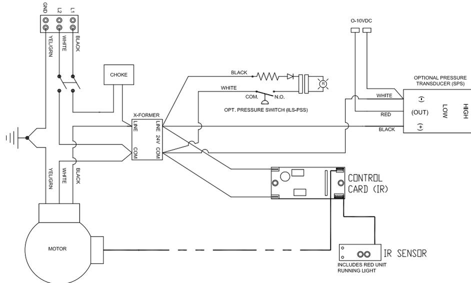
**Infrared Control Card Wiring Diagram**
