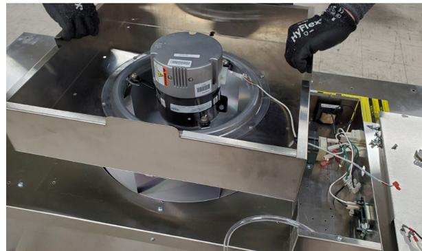
**Optional Step.** Remove the six mounting screws to free the motor/blower assembly from the pre-filter bracket..
