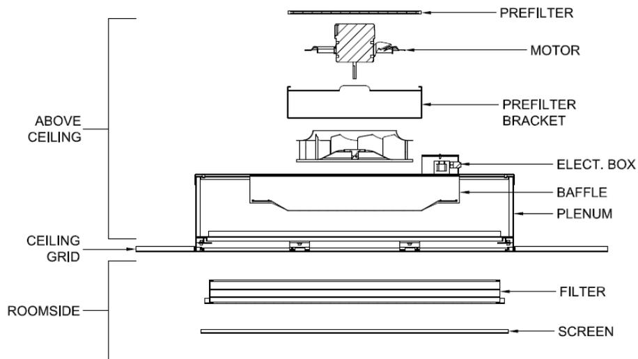
Room-side filter configuration above. The screen and filter can be removed from the room-side. All other components are only accessible from above the ceiling.
