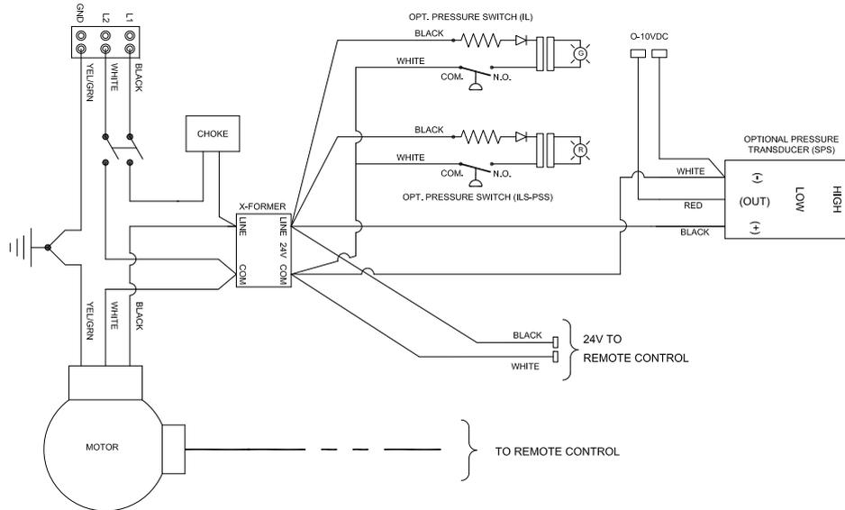
**Remote Visual Control Card Wiring Diagram**
