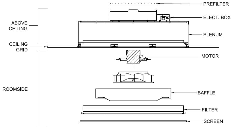
Room-side filter and motor configuration above. The screen, filter, baffle, and motor assembly can be removed from the room-side. All other components are only accessible from above the ceiling.
