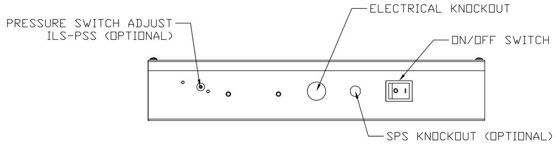
**Infrared Control Card Electrical Box Face**
