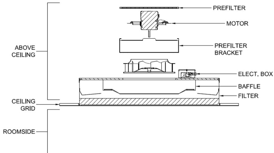
Standard filter configuration above. All components are only accessible from above the ceiling.
