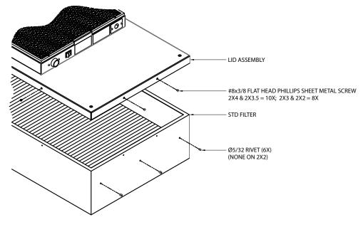
Figure 4: Standard Filter Replacement
