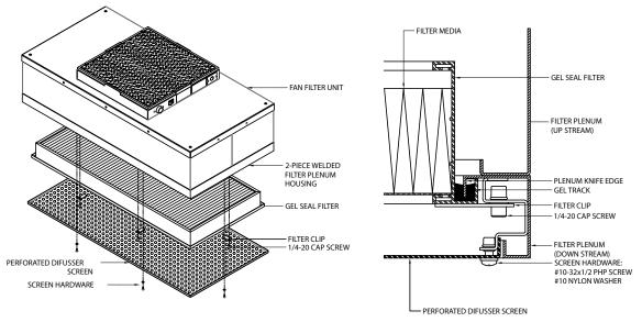
Figure 5: RSRE Filter Replacement
