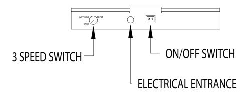
Figure 8: 3 Speed Switch Adjustment
