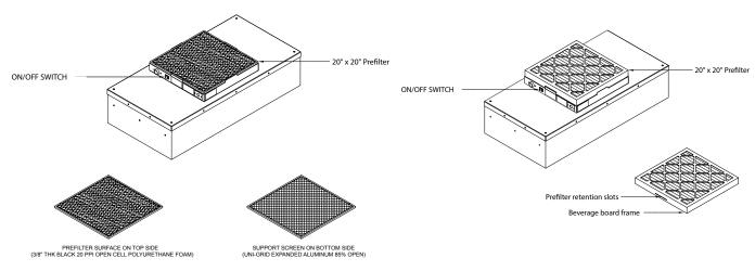
**Figure 2: Foam Cleaning Prefilter**
