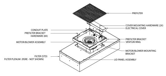
Figure 6: Standard/RSR Motor Replacement
