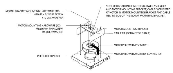
Figure 7: RSRE Motor Replacement
