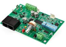
Typically the Universal Control Card (UCC) is powered inside the fan filter unit electrical box and fan filter units are daisy chained with CAT5 cabling. The UCC allows for speed control, RPM monitoring, and monitoring of the two analog inputs if used.
