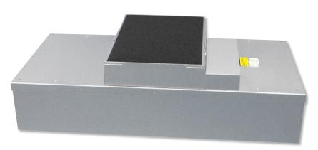
The MAC 10<sup>®</sup> IQ FFU uses a combination of EC motor technology with ENVIRCO's unique baffling system and forward curve fan to make it intelligent and energy-efficient. The electronically commutated (EC) motor with internal micro-computer provides low energy consumption (235 watts at 90 fpm (0.45 m/s)), high performance and long motor life. The IQ utilizes ENVIRCO's VE5 baffling technology, offering low sound levels that are a MAC 10<sup>®</sup> family benchmark.
