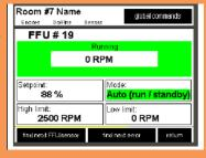
limits). Mode: setpoint and limits can be set by touching the relevant box. AC fan control screen is the same without the RPM monitor.
