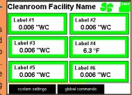
rooms are within acceptable range. The fan-blade provides FFU status (color code) and access to the facility group screen. The data file icon demonstrates the status of the datalog process. System and global settings are also easily accessible from this point.
