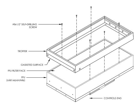
NOTE: 2X4'S SHALL HAVE THE CONDUIT CONNECTION MOUNTED ON THE CONTROL END. 2X2'S SHALL HAVE THE CONDUIT CONNECTION ON THE OPPOSITE END.
