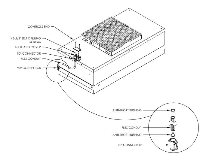
NOTE: 2X4'S SHALL HAVE THE J-BOX MOUNTED ON THE CONTROL END. 2X2'S SHALL HAVE THE J-BOX MOUNTED ON THE OPPOSITE END.
